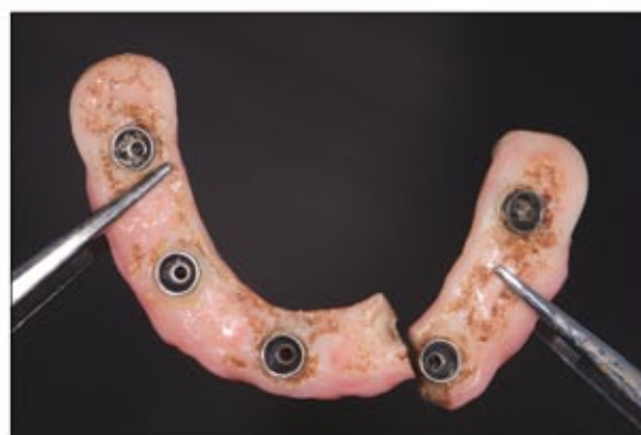
Figure 7. Fractured framework through titanium cylinder.
