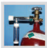
Carbon Dioxide Tank with apparatus attached to form solid Carbon Dioxide stick 4
